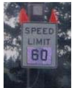
Variable Speed Sign
